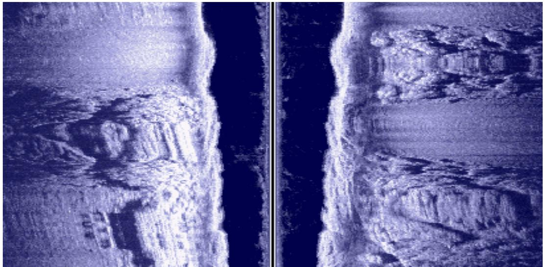
Figure 2: Humminbird sidescan sonar image used to determine the location of sampling locations on sand immediately adjacent to rocky reefs. Smooth areas are sand and rough areas are reef.
