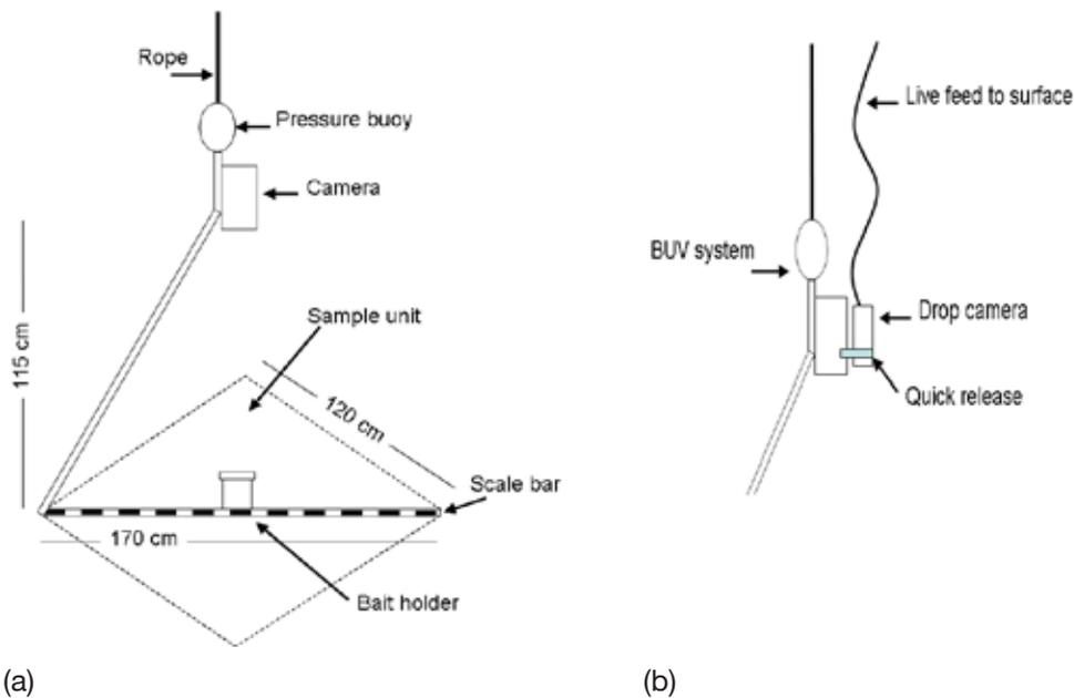
Figure 1: Baited underwater video system (BUV). (a) This system sits on the substrate and is kept upright by a pressure buoy. The camera films fish attracted to the bait. (b) A quick release camera supplying real time footage to the surface is attached allowing the baited underwater video to be placed in complex habitats such as kelp forests and rocky reef systems. The umbilical camera is removed once the baited underwater video is in place.
