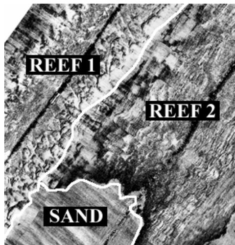
**Figure 4:** A section of a reef system located within the Te Angiangi reserve clearly showing different physical habitat types. Note that dark straight lines are the midpoints of the side-scan sonar sweeps.
