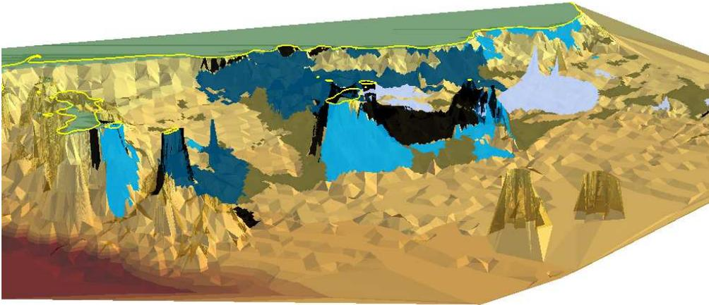
**Figure 4:** Three dimensional view of the bathymetry, with the sedimentary facies observed within the reserve overlain. ■ The sand facies within the reserve are shaded yellow depending on depth. ■ Black- areas were not covered by side-scan, ■ dark blue = Rock-sand matrix (RSM), ■ blue- Bedrock/sand, ■ lilac = Flat rock-sand (FRS), ■ green = Megarippled gravely sand (MGS). Maximum depth is 20m.
