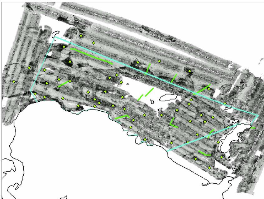
**Figure 2:** Side-scan produced by University of Waikato for the Department of Conservation. Sampling positions are marked by dots (10 min drop camera positions) and lines (camera transects).
