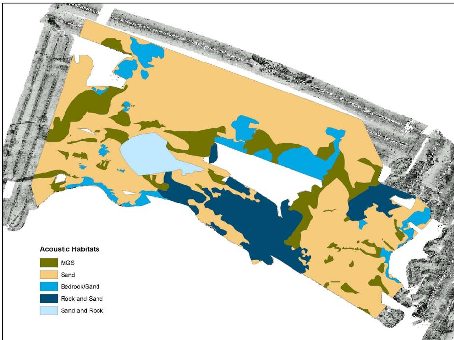
**Figure 3:** Acoustic habitats related to sedimentary facies, within the reserve, identified from the side-scan imagery, overlaying the side-scan. The “Rock and Sand” vs “Sand and Rock” habitats reflect the dominance of rock and sand respectively.
